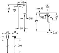
Touch: setting the sensor or features, by touching the sensor 6V Lithium CRP 2 - life time up to 4 years Battery: Mains operation: plug-in transformer 100-250VAC / 6VDC;
