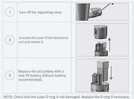
ATTENTION: Dry the inside of the cover and interior of the flush valve body carefully. The interior of the flush valve body and the cover plate with the electronic cap must be fully dry before reassembling the parts.
